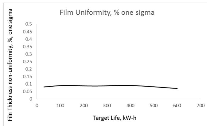
Figure 11. Film properties of AlScN deposition as a function of target life
