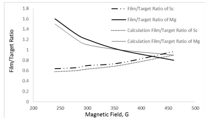
Some mismatch between calculated and actual film/target composition ratio versus magnetic field could be considered as an error for different scattering shape for different type of dopant (heavier atoms, normally at given target voltage, have broader scattering and some material is losing due to deposition on shields. Lighter atoms, at given target voltage,
